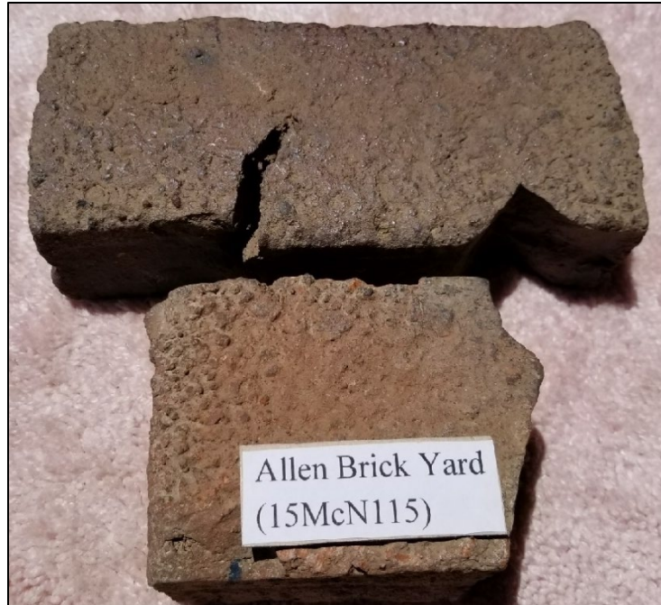
Figure 8. Two common bricks from the Allen Brick Yard Site that may have been rained on prior to firing. The top brick is SP-7 and the bottom brick is SP-17.
