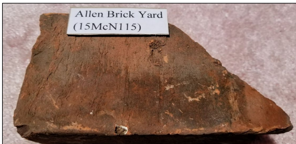
Figure 4. Common brick struck across the short axis from the Allen Brick Yard Site (Specimen SP-15). Note the strike lines across the short axis of the brick.
