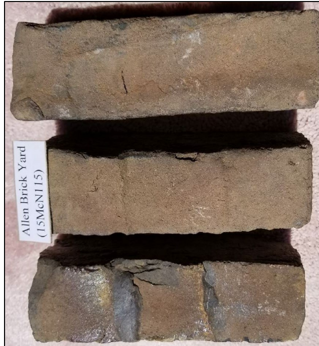
Figure 5. Side-view of the common bricks from the Allen Brick Yard Site. The top brick (SP-8) has a length-wise stacking impressions. The center brick (SP-1) has cross-wise stacking impressions. The bottom brick (SP-2) has portions of adhering bricks that fused during the firing process.
