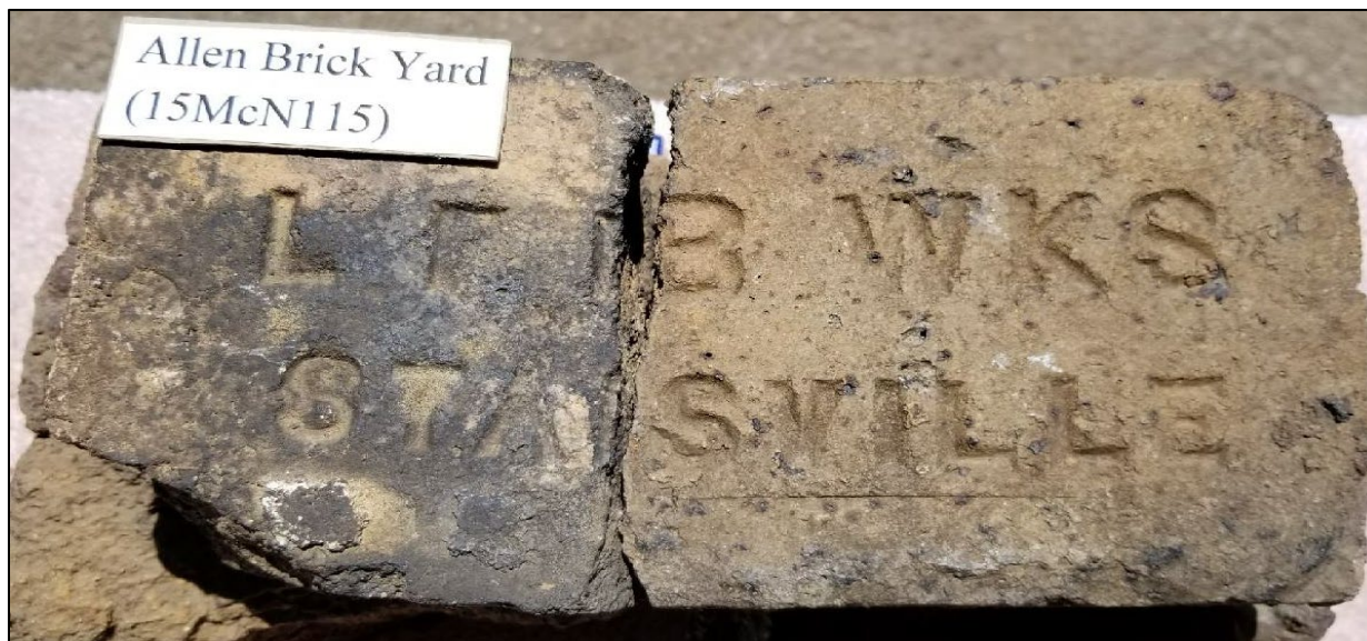
Figure 9. Two fragmentary fire bricks from the Allen Brick Yard Site. On the left (SP-20) is a LFB WKS/STANDARD Fire Brick and on the right (SP-18) is a LFB WKS/LOUISVILLE Fire Brick.
