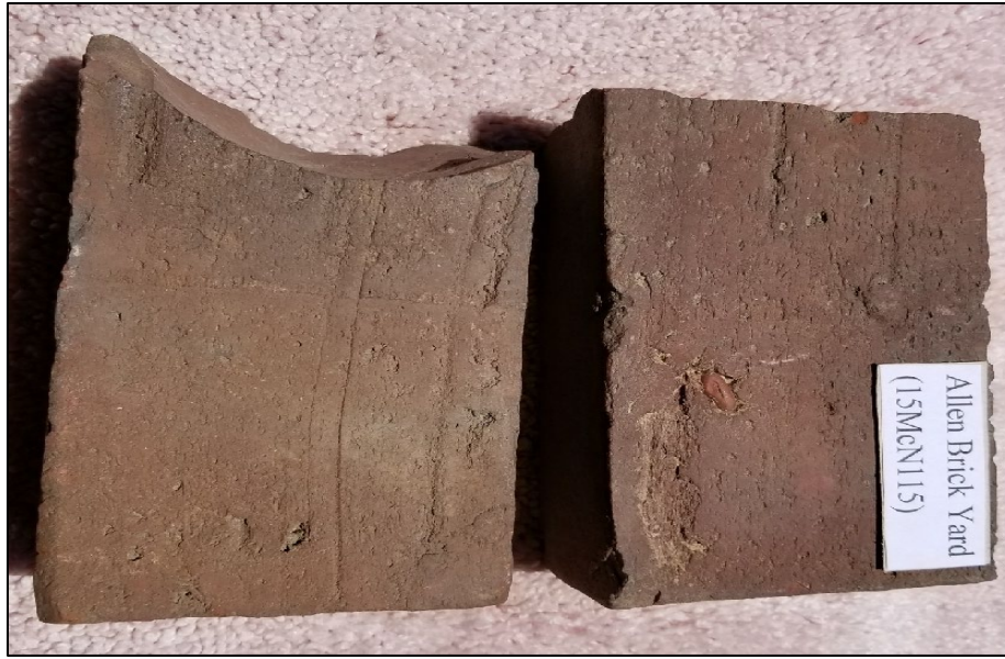
Figure 2. Two dense, well-made bricks from the Allen Brick Yard Site. The top brick is specimen SP-2 and the bottom brick is specimen SP-13. Note the strike lines running length-wise.
