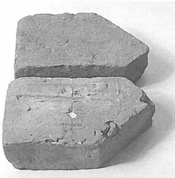
Figure 9. Two Soft-Mud Cornice Bricks From 15 McN114. The upper specimen shows the sandy surface opposite the strike while the lower specimen shows the struck surface.
