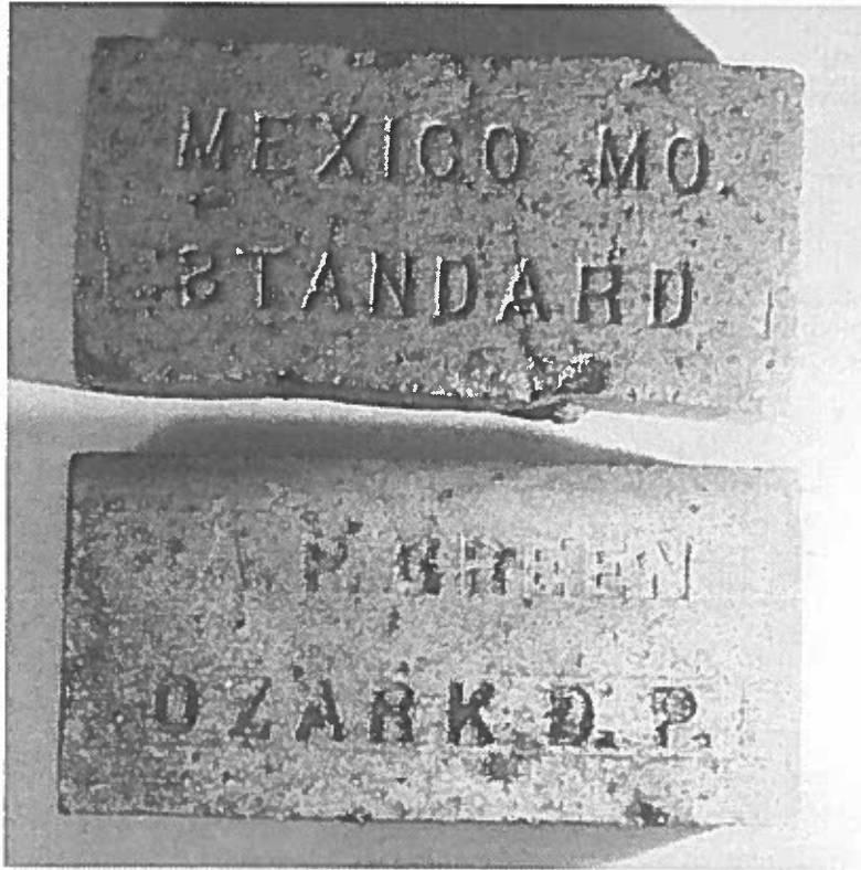
Figure 20. Missouri Fire Brick Brands: MEXICO MO./STANDARD (Specimen L-6) and A. P. GREEN/OZARK D. P. (Specimen G-3).
