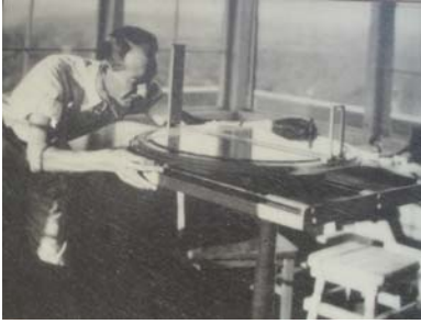
Alidade at Bald Rock Lookout Tower. From USFS Interpretive Marker at Bald Rock Tower site.
