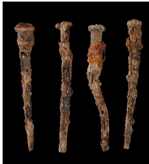
Top Almost all of the Cemetery's wooden coffins were constructed with late machine-cut nails.
