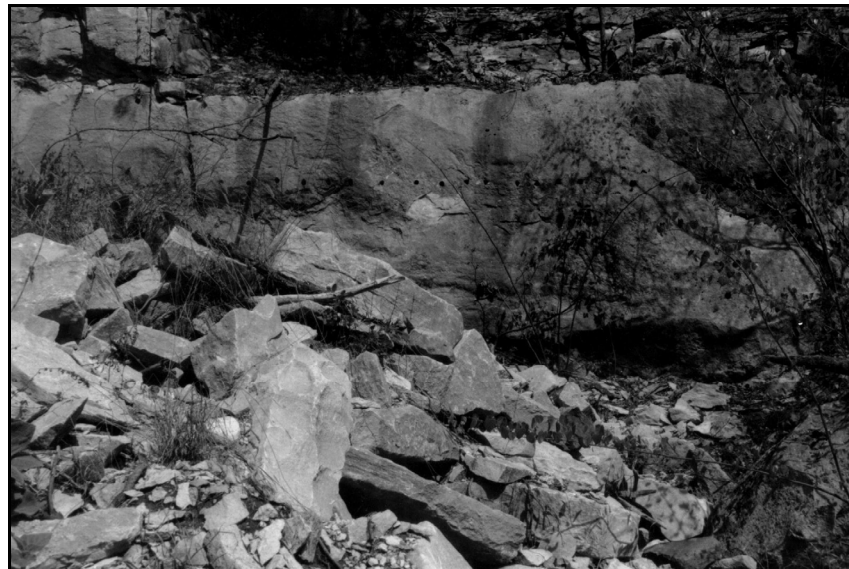
Figure 9. Eastern Working Face of the Shrull Quarry With Stone Rubble in Foreground (Note the drill hole scars across the top of the rock ledge and the row of complete drill holes located horizontally across the center of the rock ledge).
