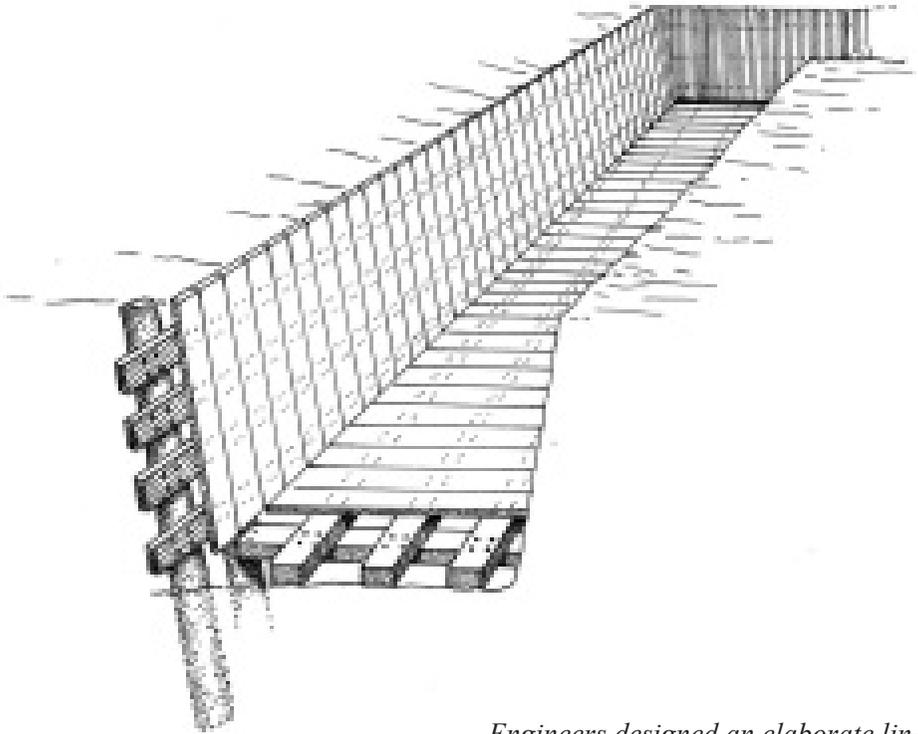
*Engineers designed an elaborate lining made of oak planks to protect the Yellow Creek Canal.*
